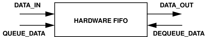
Figure 2.19 An interface model of a hardware FIFO.
