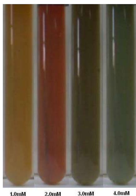
Figure 3. The final colour of Ag nanoparticles solution as a function of ascorbic acid concentrations.
