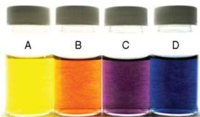
Figure 2. Optical images of the aqueous dispersions of the silver nanoprisms of four different sizes. The letters are the same as given for the absorbance spectra (Figure 1).
