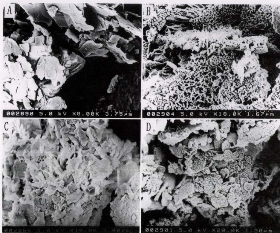
FIG. 3. Scanning electron micrographs of the synthesized smectites from some clays.
