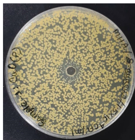
FIGURE 9: S. aureus bacterial zone of inhibition by the produced CuO NPs at a dosage of 70 \mu\text{L} with concentration of 100 \text{ mg/L} .
