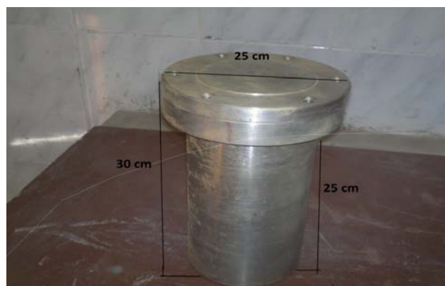
Figure 1. Schematic of the a Teflon-lined stainless steel autoclave
