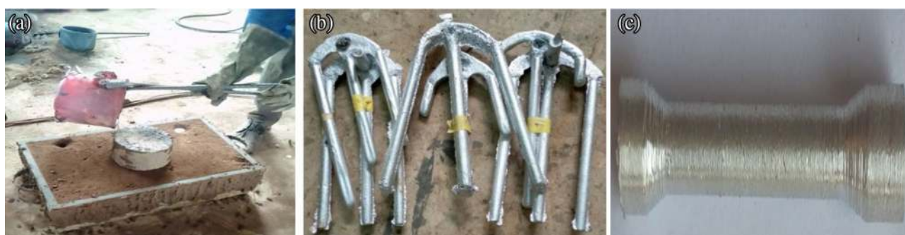
Figure 2. (a) Pouring of molten metal composite into prepared sand mold (b) solidified metal composite (c) tensile test sample.
