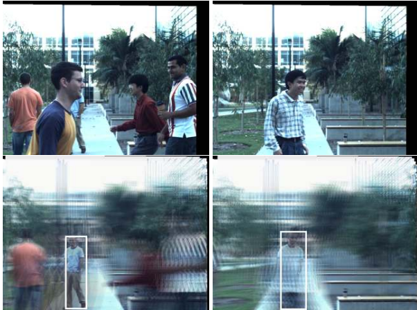
Figure 7. Tracking a person in a crowd. The person in a single camera is significantly occluded by different people in the group (top row). Using Non-Linear TTO we can track the person successfully (bottom row).
