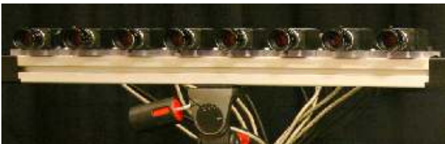
Figure 5. Our array of 8 VGA resolution video cameras.
