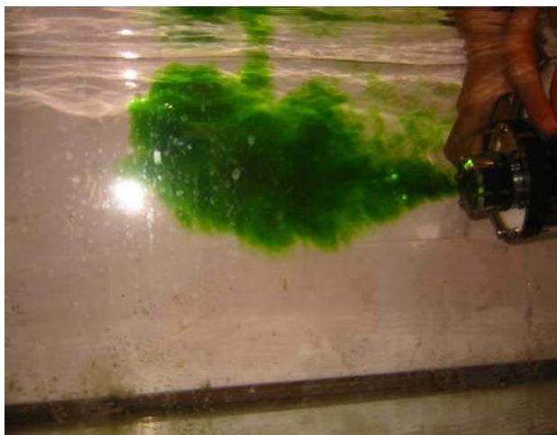
Fig. 7. Dye flow visualization of synthetic jet thruster operation.
