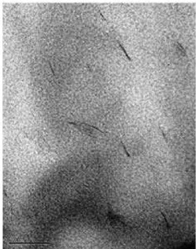
Figure 5. PA-6 melt compounded with 1.14 wt% of organoclay: (from top to bottom) Cloisite ® 15A, Somasif MAE, and Lucentite SAN. The TEM magnification is the same, 200k (see the 100 nm scale bar). 102
