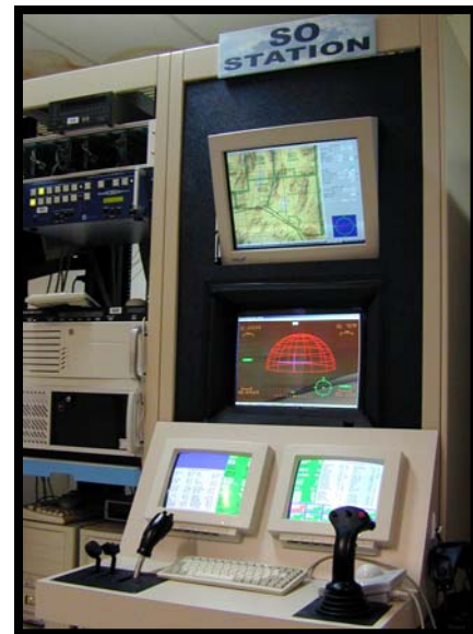
Figure 7. UAV sensor operator control station.
