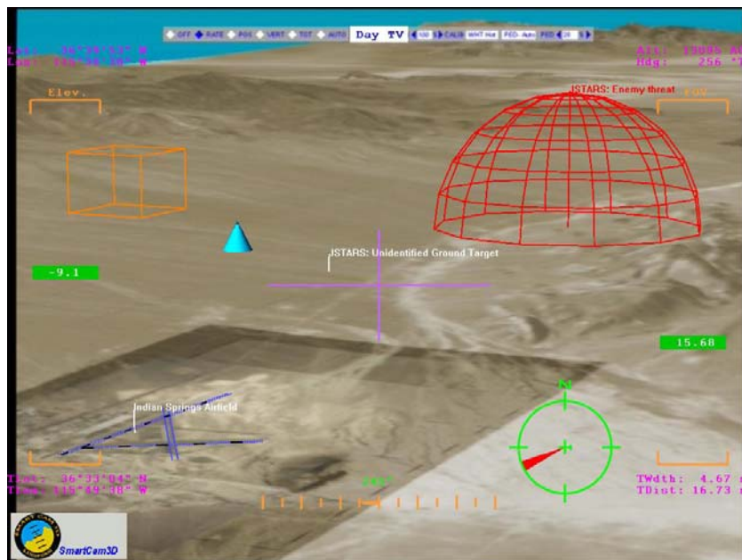
Figure 3. Synthetic vision symbology added to simulated UAV gimbal video imagery (symbology marking threat, landmarks, areas of interest and runway).
