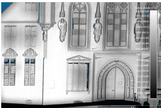
Fig. 5. The resulting mesh of the building with a medium amount of highly reflective surfaces.
