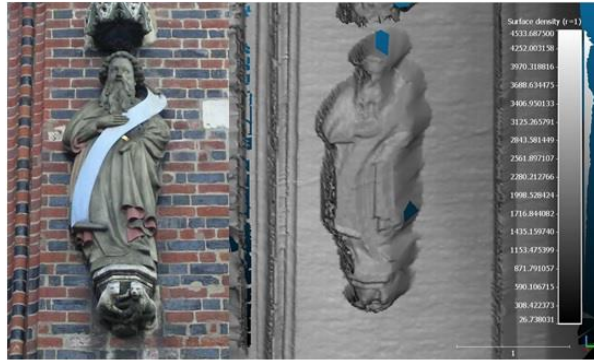
Fig. 7. A feature on the façade (left) and the constructed mesh (right).
