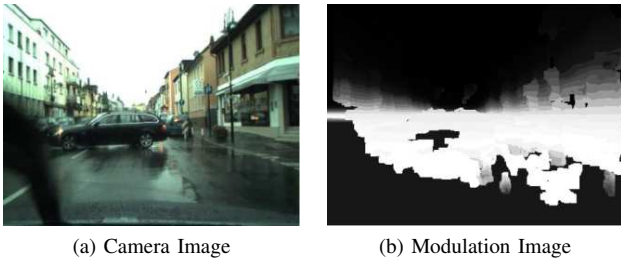
4: A typical modulation image (b) used for incorporating scene context into detection algorithms. Light values in the modulation image relate to plausible locations for vehicles in the image (a), dark values to implausible ones.
