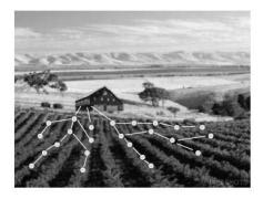
It depicts a precision agriculture deployment—an active area of application research. Hundreds of nodes scattered throughout a field assemble together, establish a routing topology, and transmit data back to a collection point. The application demands for robust, scalable, low-cost and easy to deploy networks are perfectly met by a wireless sensor network. If one of the nodes should fail, a new topology would be selected and the overall network would continue to deliver data.
