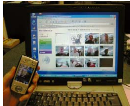
Figure 1: UI sharing between a cell phone and a laptop computer, across a short range wireless link.
