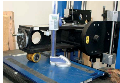
7: Measurement of SW deformation properties on static adhesor (authors)
