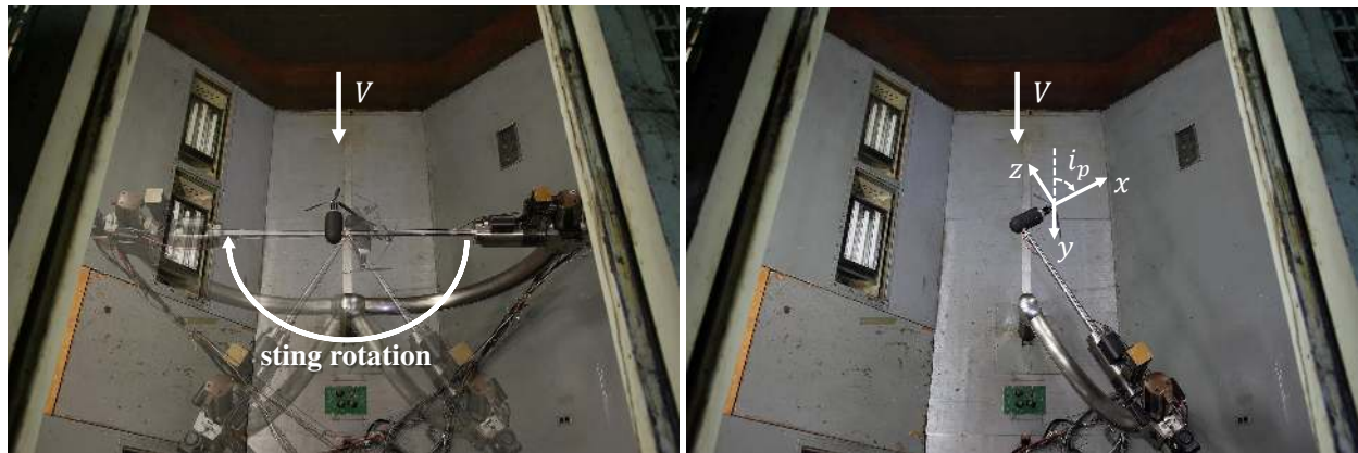
(a) Multi-exposure image of a propeller wind tunnel run
