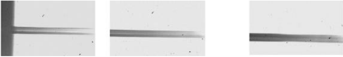
Figure 8. Magnified image of 50 micron diameter liquid xenon filament jet (First frame at pinhole exit, second frame 2 mm downstream, third frame 8 mm downstream)
