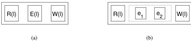
Figure 4.16: (a) PE2 and PE3 with pipelined R , E , and W units. (b) E unit is further refined to have more pipelined execution units.
