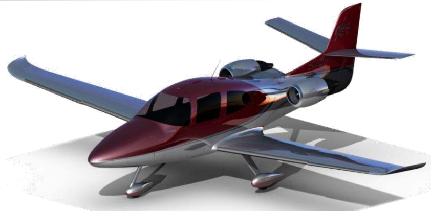
Concept airplane used in this study is a jet-powered variant of Cirrus Aircraft's propeller-driven SR22
