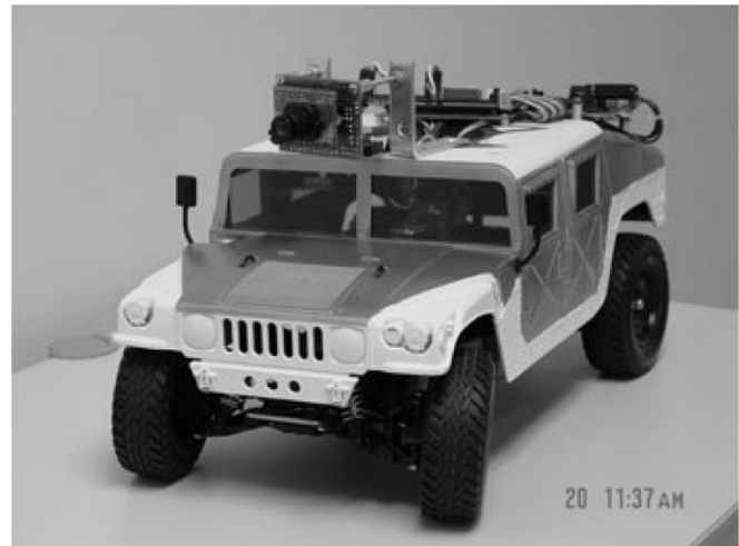
Fig. 5. Student project using the small hobbyist R/C Hummer vehicle with the color tracking CMUcam all controlled by the Altera Nios SOPC board.
