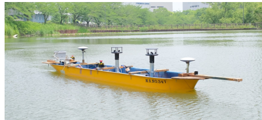
Fig. 3: Scale Model Ship of Esso Osaka
