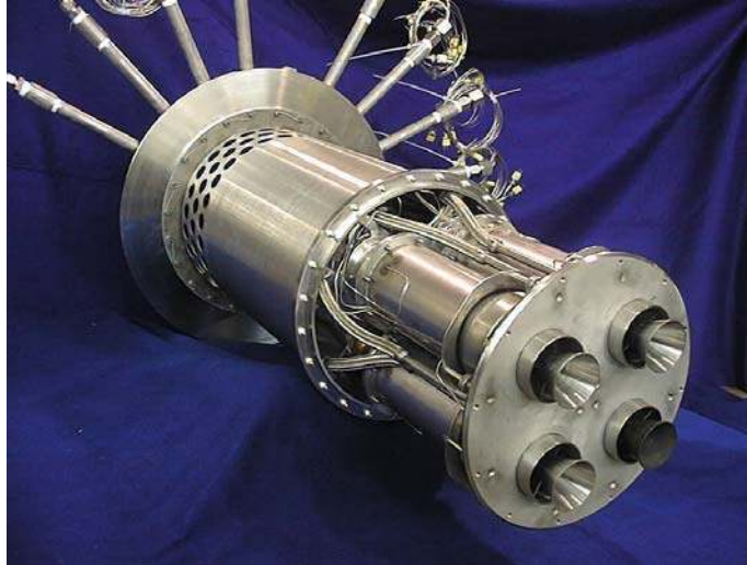
Figure 2.1.14. Photograph of four-RCL-injector assembly, prior to installation in Saturn engine.
