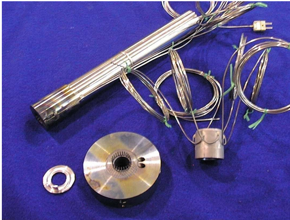
Figure 4-1. Photograph of sub-scale catalytic reactor for syngas combustion.
