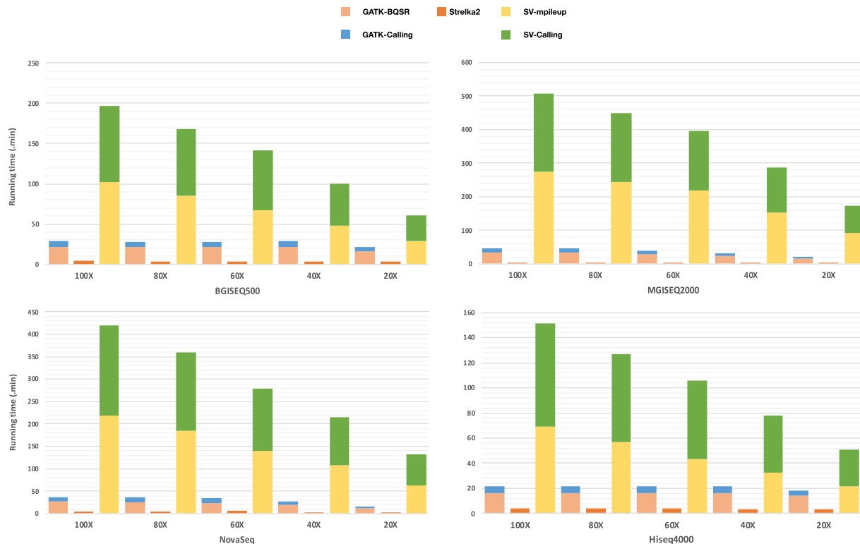
Figure 4. Variant calling runtime of multiple combinations in WES datasets. The variant calling runtime of each combination run on a Tianhe-2 supercomputer with 24 virtual CPUs and 88 GiB of memory. All combinations were configured to schedule tasks over all 24 virtual CPUs. The coverages of the down-sampled datasets were approximately 20X, 40X, 60X, 80X, 100X, respectively. Among them, variants calling in SK2 sets 24 threads, GATK used the default setting thread in BQSR and 24 threads setting in variants calling, and SV used the default setting thread in mpileup and variants calling.
