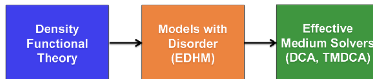
Figure 28. Organization of the modular approach to first-principles calculations of localization. A DFT of the pure system and a DFT supercell calculation of a single impurity are performed as the first step. In the second step, the EDHM converts the DFT output into model parameters of the disordered system. In the third step, the TMDCA is used to study the materials-specific localization properties.
