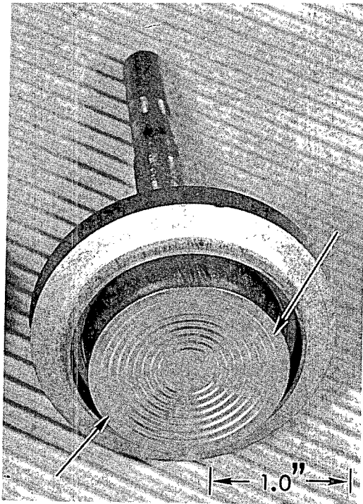
(a) Cracks (arrows).
