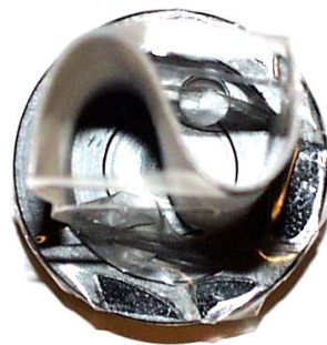
Figure 2. Top view of polyethylene sheet folded into an ‘S’ shape. The polyethylene was held in place using scotch tape. The sample was mounted such that the THz beam was in the plane of the paper and the sample was rotated about the z -axis (the axis pointing out of the page).
