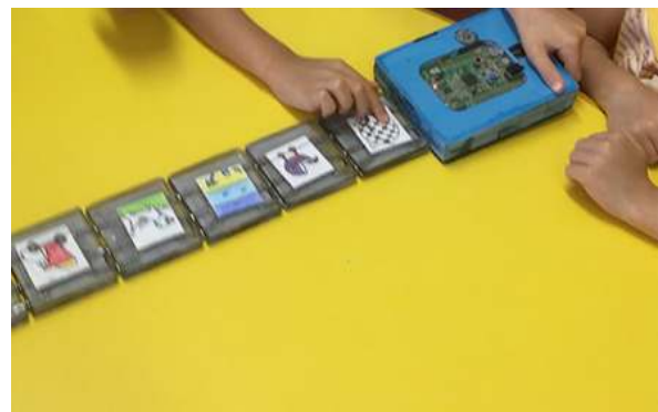
Figure 6. Children playing the recorded audio sequence by connecting the clients to the server.
