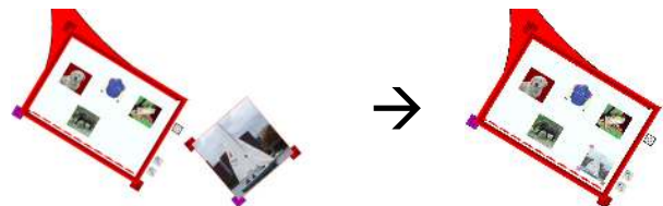
Figure 8. An object is moved from the tabletop to an ancillary display by dragging it onto a WIM view. The orientation of the object is corrected once it is placed on the vertical display.
