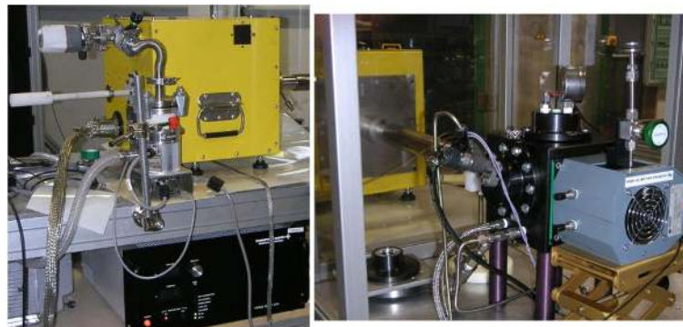
Figure 1. Experimental setup, inset a) illustrates the injector nozzle. Photo on the left shows the flash X-ray source, and photo on the right details the spray chamber (black) equipped with the X-ray camera
