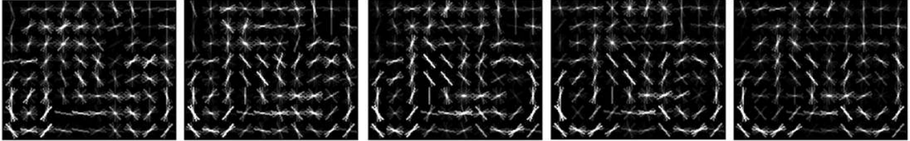
Figure 3. Bicycle classifiers learned using a motorbike classifier as the source and with an increasing number of samples (1,3,6,9,20) from left to right. Note the transition from a template that looks like a motorbike (left) to one that looks like a bicycle (right). A-SVM method is used for learning.
