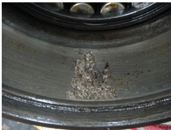
Figure 17. The spall fault on the outer race.
