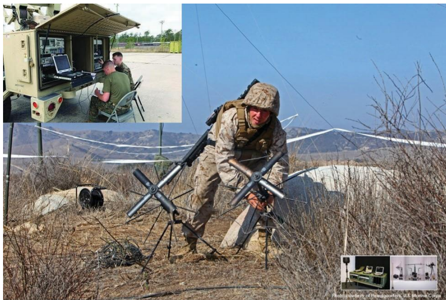
Figure 3.1 A Marine Sets Up a Tactical SIGINT Collection System
