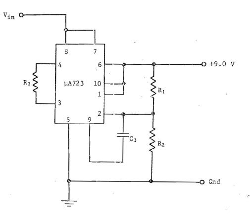
At 12 V input and load current of 1 mA the power input is 30 mW.
