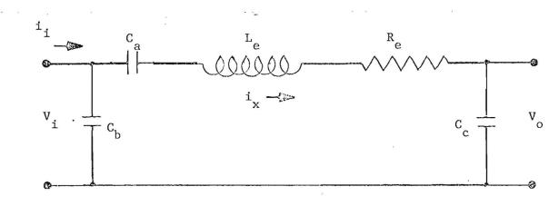
Figure 1. Equivalent Circuit of the Pi Network at the Resonant Frequency
