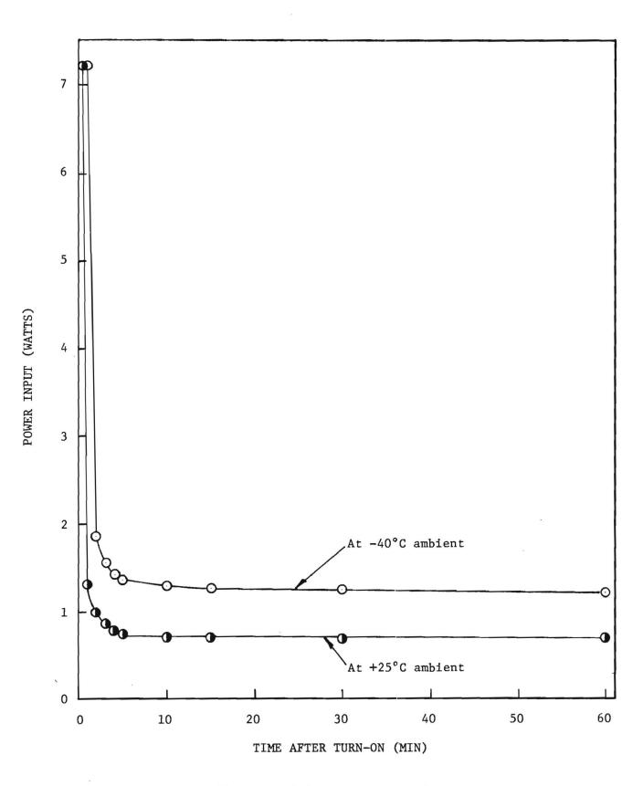
Fig.29. TMXO-2 input power requirements.
