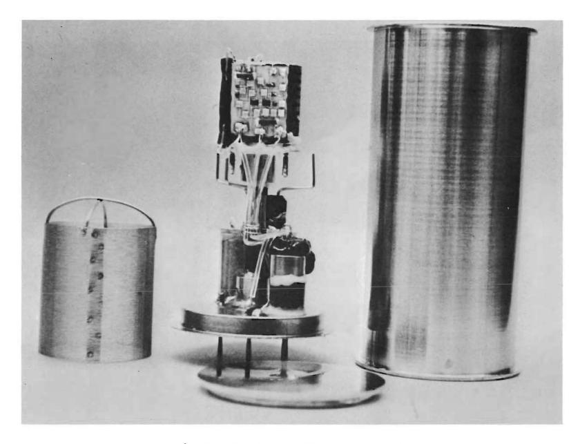
Fig. 8. TMXO No. 3 before NRC-2 and cap installed.
