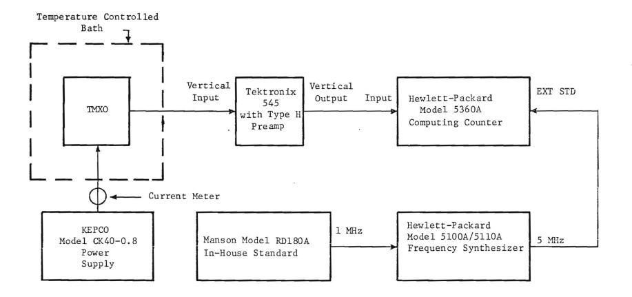
Fig.19. System for the measurement of warmup time, warmup power and the frequency during and after warmup. Frequency readout is digital.
