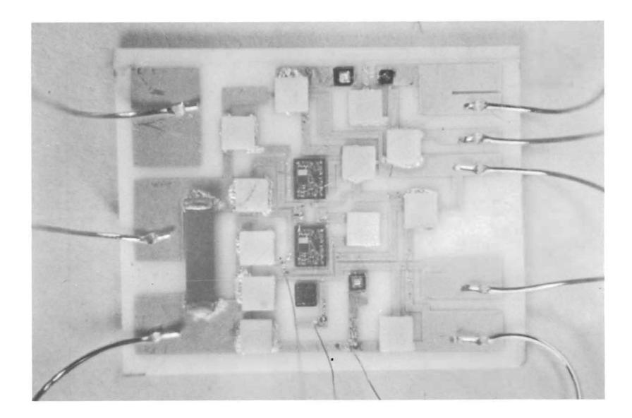
Fig. 16. Photograph of hybrid temperature circuit board.
