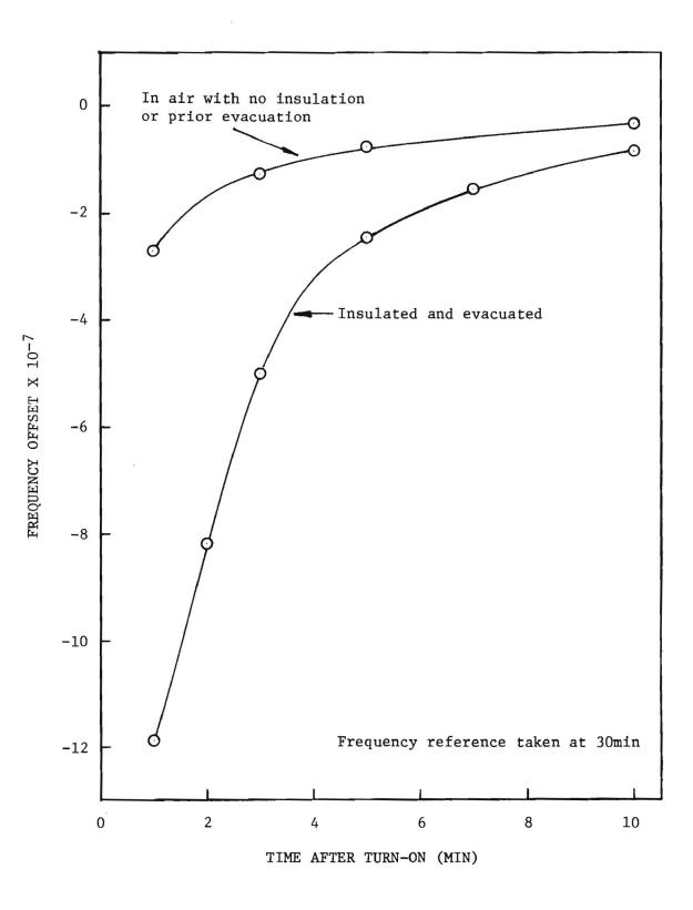
Fig. 23. TMXO-1 warm-up comparison at +25°C ambient before and after encapsulation.
