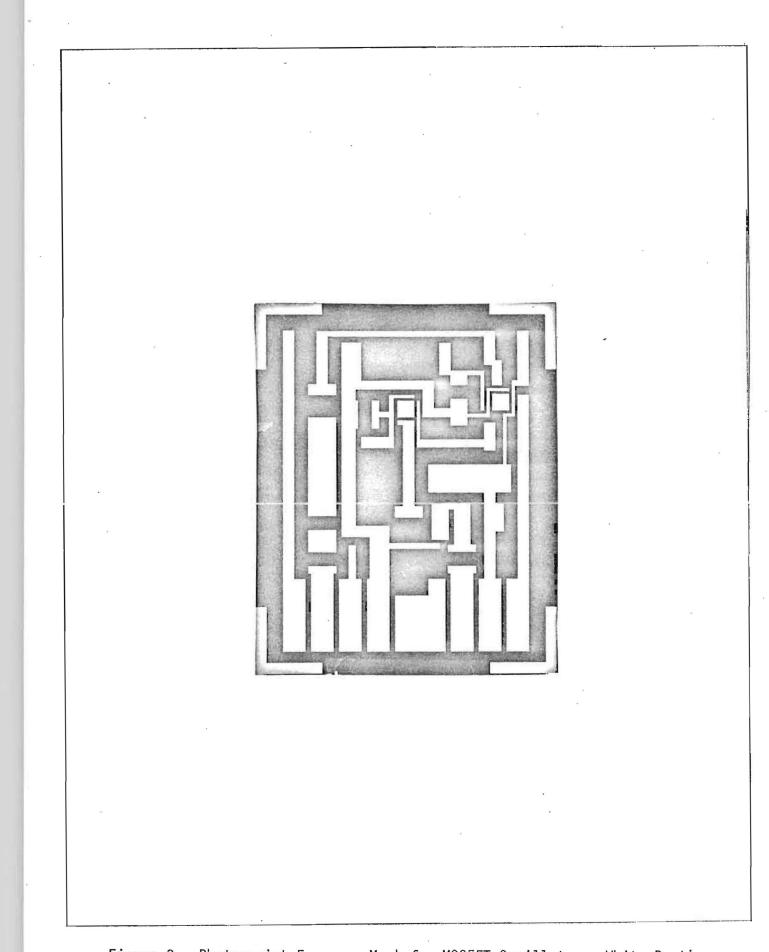
Figure 3. Photoresist Exposure Mask for MOSFET Oscillator. White Portions are Cr + Au Conductors. Scale: 6X.
