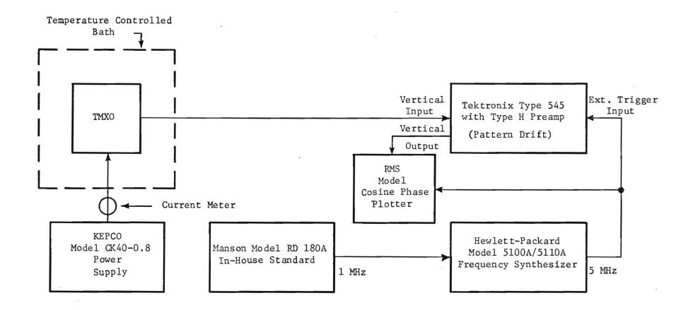
Fig. 20. Alternate system for making performance measurements. The frequency readout is analog. This method especially suited for long periods of operation with equipment unattended.
