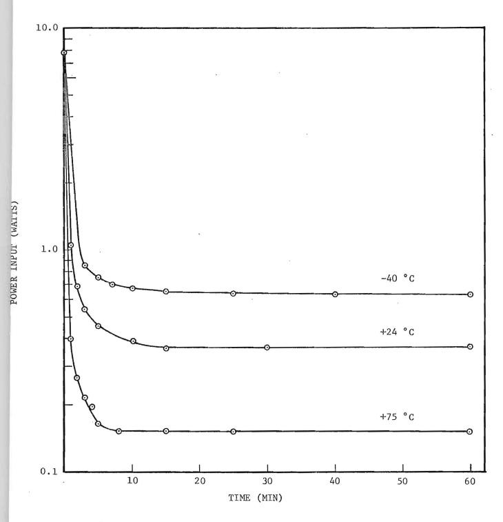
Fig. 4. Total operating power vs time for operating TMXO Model No. 1 in different ambient temperatures.
