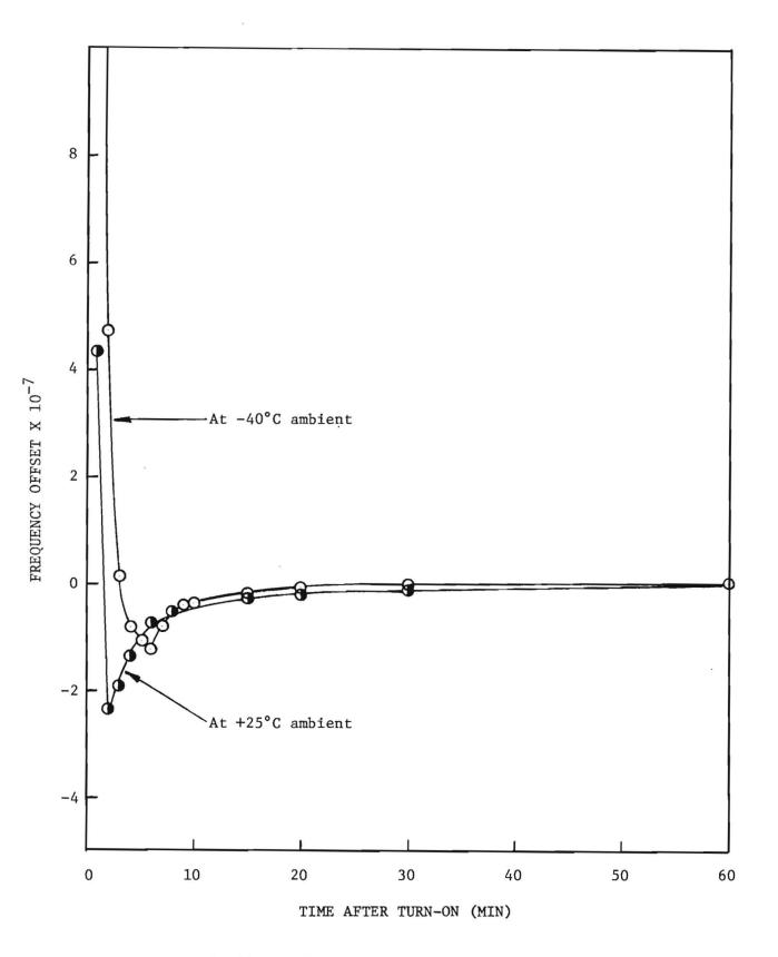
Fig.32. TMXO-3 warm-up after encapsulation.
