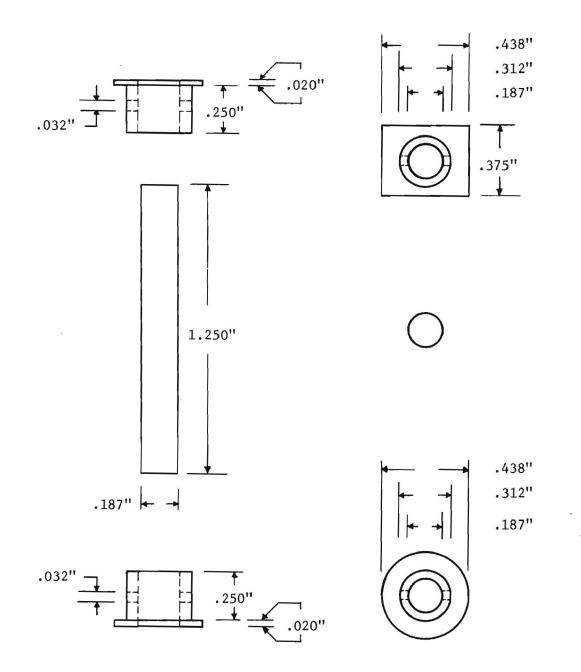
Fig. 7. Support pedestal assembly for TMXO Models Nos. 2 and 3.
