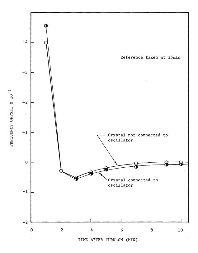
Fig. 28. TMXO-2 warm-up showing effect of oscillator circuitry.
