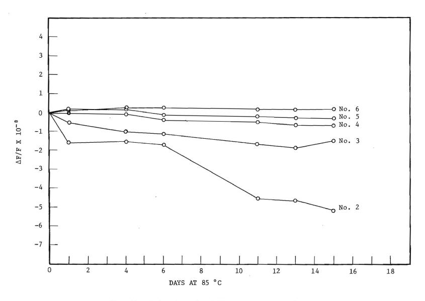
Fig. 19. Aging data for 5 MHz resonators purchased for the tactical miniature crystal oscillator.
