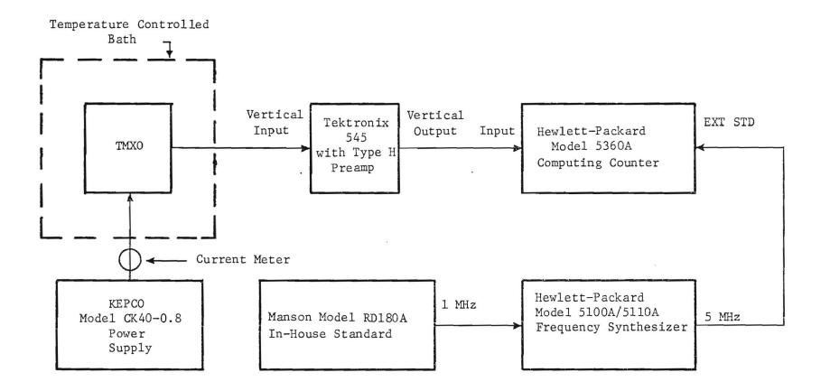
Fig. 1. System for the measurement of warmup time, warmup power and the frequency during and after warmup. Frequency readout is digital.
