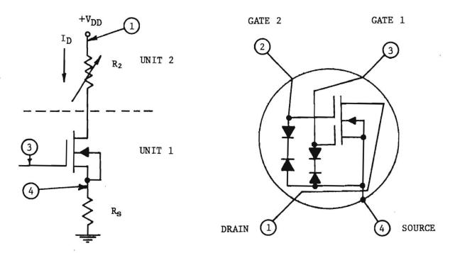
Fig. 12. Equivalent circuit representation of the two units in a dualgate MOSFET.
