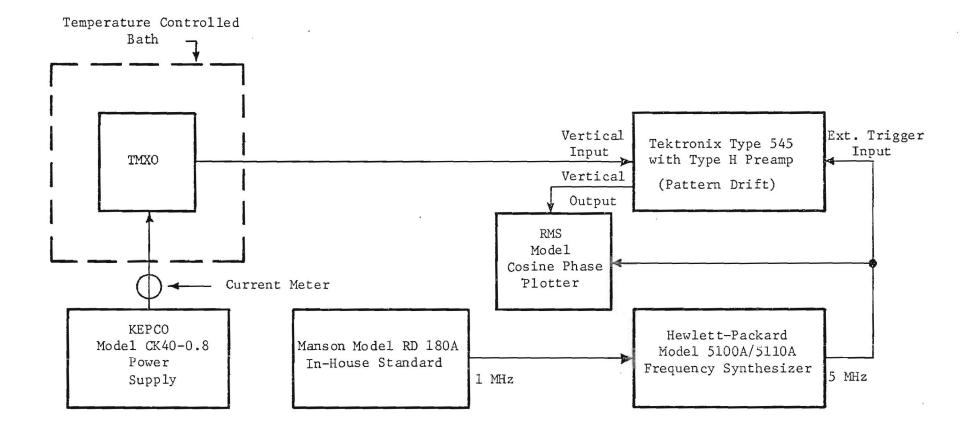
Fig. 2. Alternate system for making performance measurements. The frequency readout is analog. This method especially suited for long periods of operation with equipment unattended.
