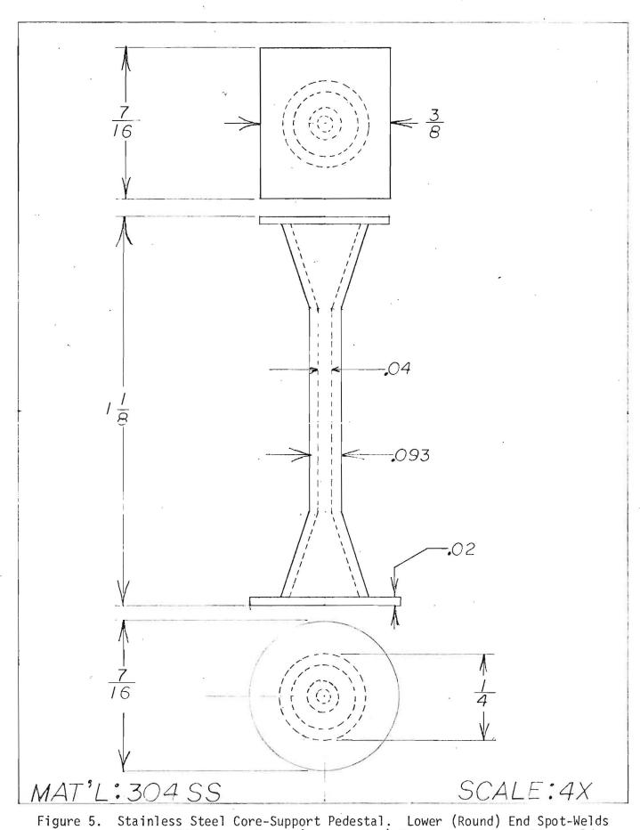
igure 5. Stainless Steel Core-Support Pedestal. Lower (Round) End Spot-Welds to Type "D" Base. Upper (Rectangular) End Spot-Welds to HC-6 Holder Flange.
