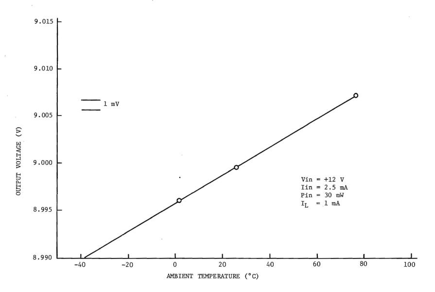
Fig. 15. Output voltage vs temperature for voltage regulator.
