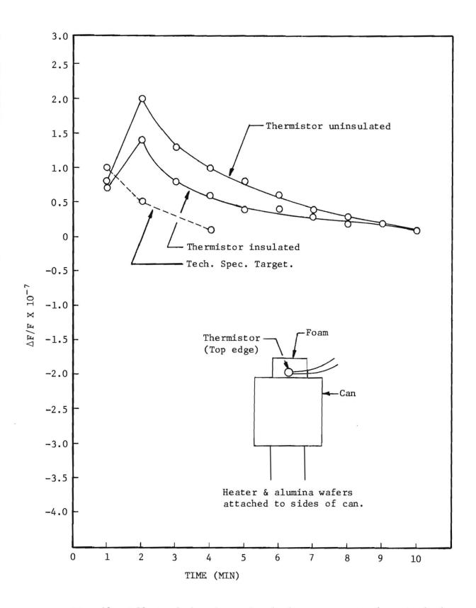
Fig. 12. Effect of thermistor insulation on warm-up characteristics.
