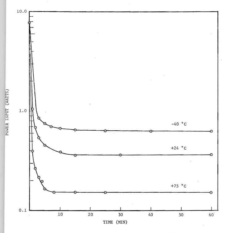
Fig.25. Total operating power vs time for operating TMXO Model No. 1 in different ambient temperatures.
