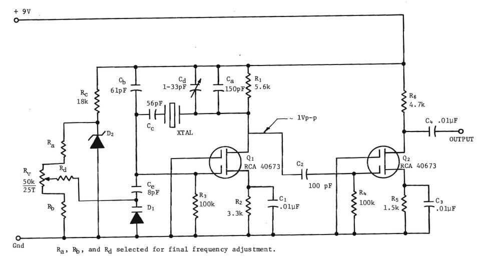
Fig. 6. Circuit diagram of the MOSFET Crystal-Controlled Oscillator.
