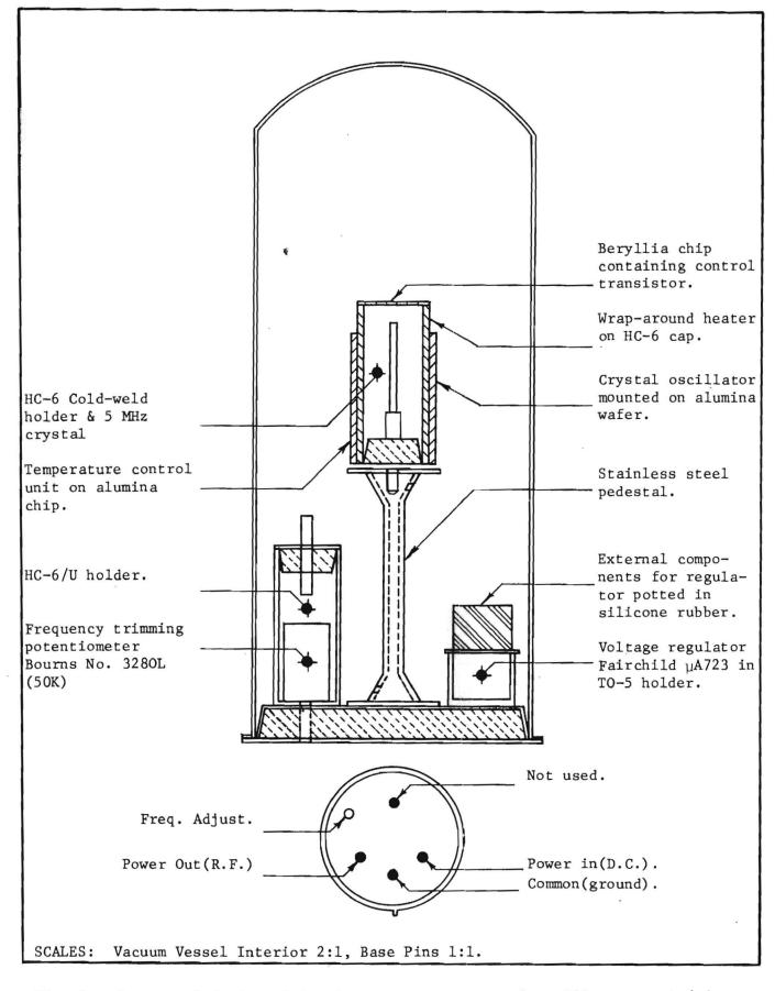
Fig. 1. Conceptual design of tactical miniature crystal oscillator mounted in a type "D" cold-weld holder.
