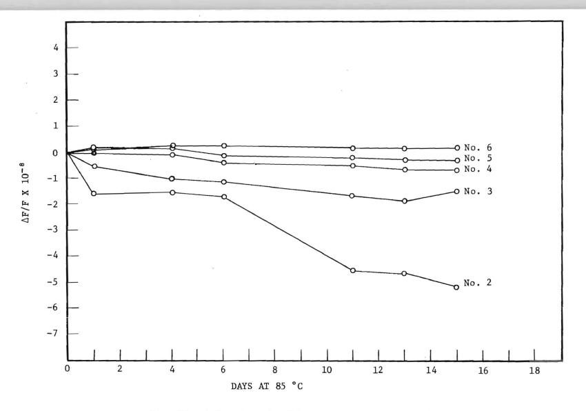
Fig. 18. Aging data for 5 MHz resonators purchased for the tactical miniature crystal oscillator.
