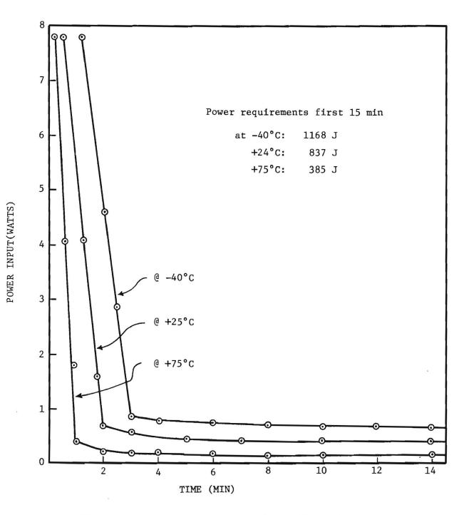
Fig. 24. Warm-up power profiles for first 15 minutes after turn-on. The technical guidelines requirement is 810 W-sec over the entire ambient temperature range.
