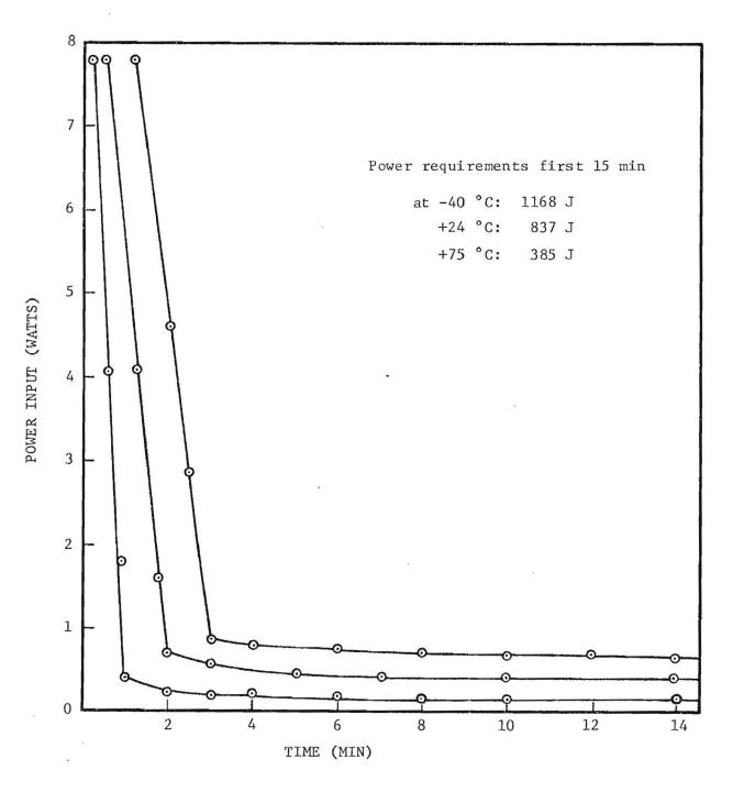
Fig. 3. Warmup power profiles for first 15 minutes after turn-on. The technical guidelines requirement is 810 W-sec over the entire ambient temperature range.
