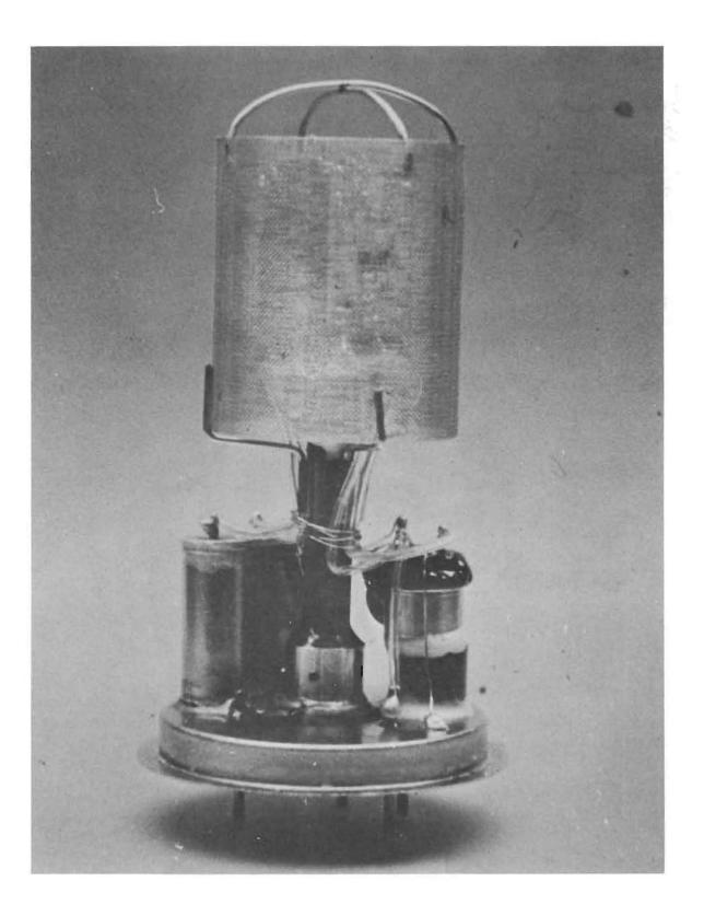
Fig. 9. TMXO No. 3 showing screen installation.
