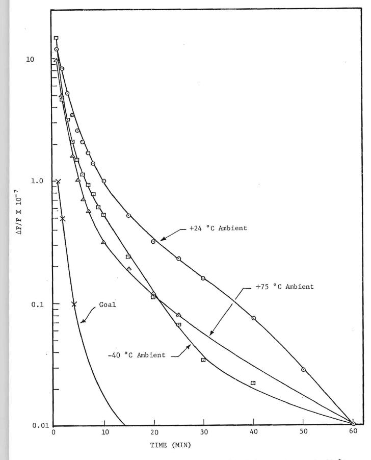
Fig. 5. Warmup time vs frequency for ambient temperatures of -40 °C, 24 °C and 75 °C.
