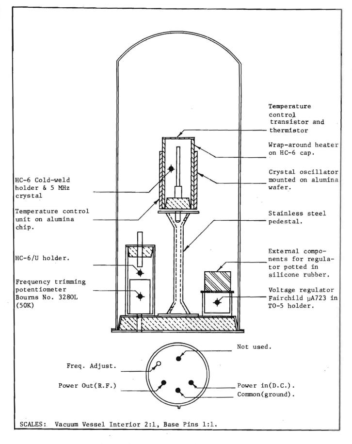
Fig. 1. Basic conceptual design of TMXO.
