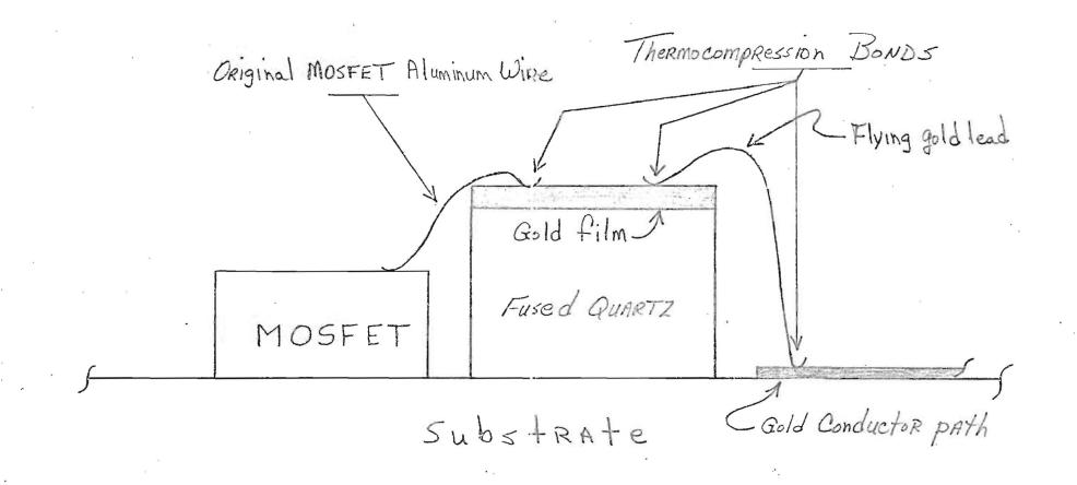
FIGURE 1: Present lead bonding technique for MOSFET Q, and Qz. All leads bonded in this manner.
