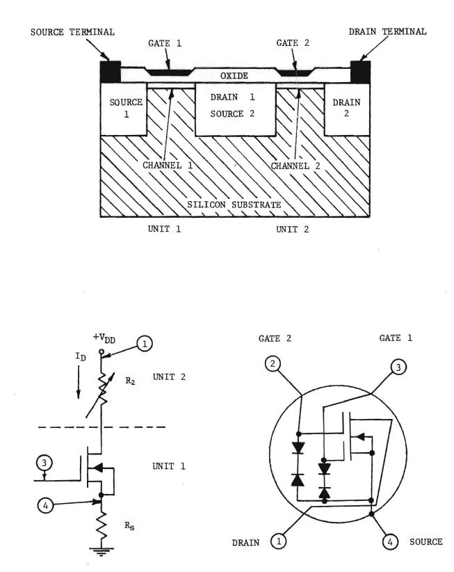
Fig. 7. Equivalent circuit representation of the two units in a dualgate MOSFET.
