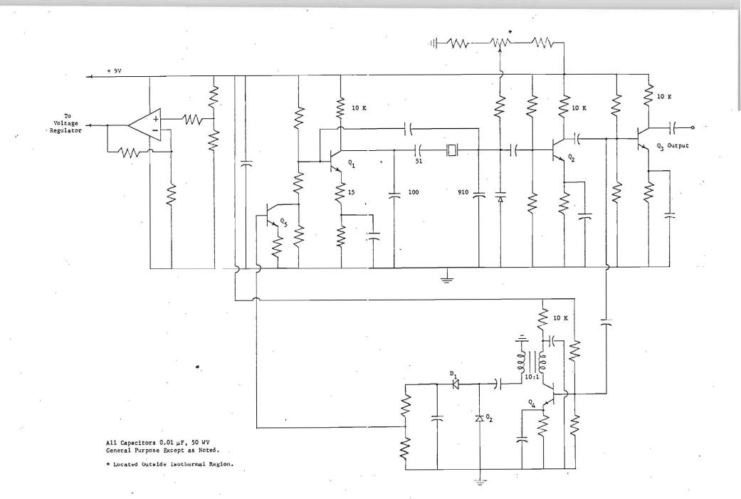
Oscillator Schematic Diagram. Figure 2.
