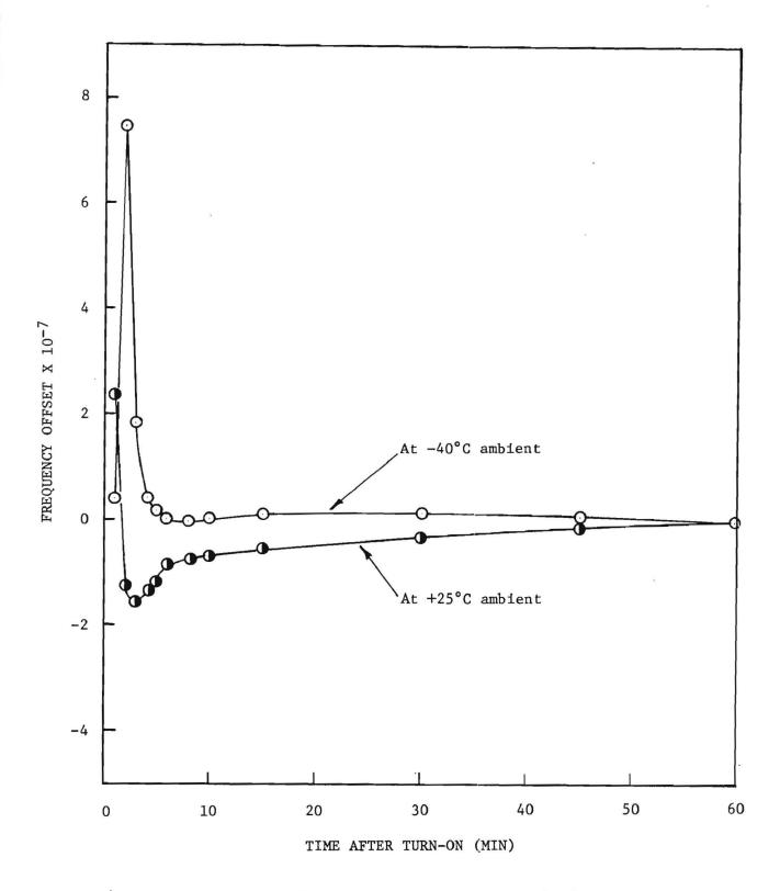
Fig.31. TMXO-2 warm-up after encapsulation.
