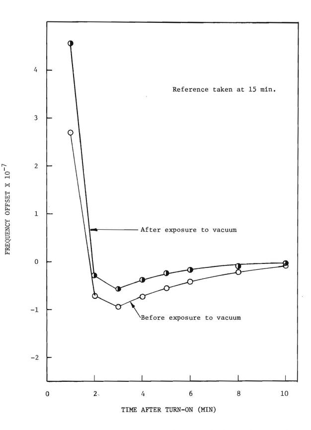
Fig.34. TMXO-2 warm-up comparison before and after unit exposed to vacuum.
