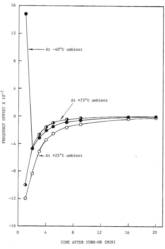
Fig. 26. TMXO-1 warm-up after encapsulation and evacuation to  ${<}1X10^{-5}{\rm torr}$  .
