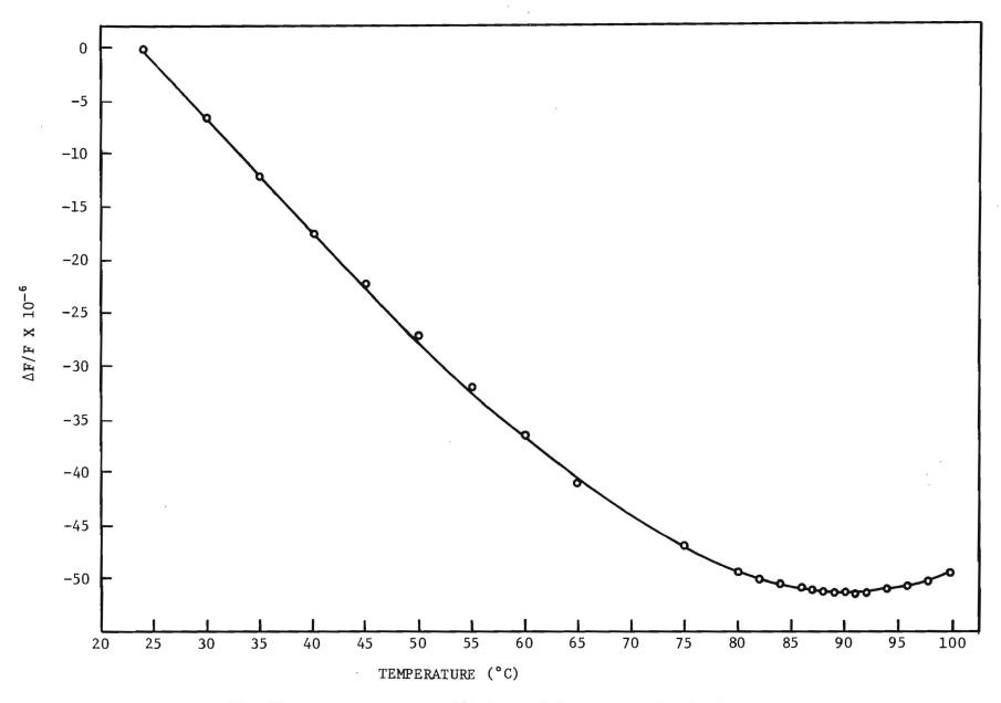
Fig. 17. Temperature coefficient of frequency of unit 6.
