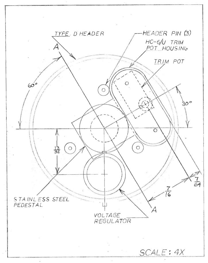
Figure 4. "Floor Plan" for the Type "D" Base. Crystal Holder on the S.S. Pedestal Positioned so the Pins are on Line A-A.
