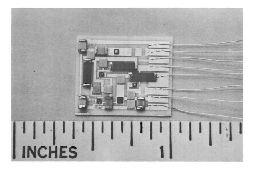
Fig. 15. Photograph of hybrid oscillator board.
