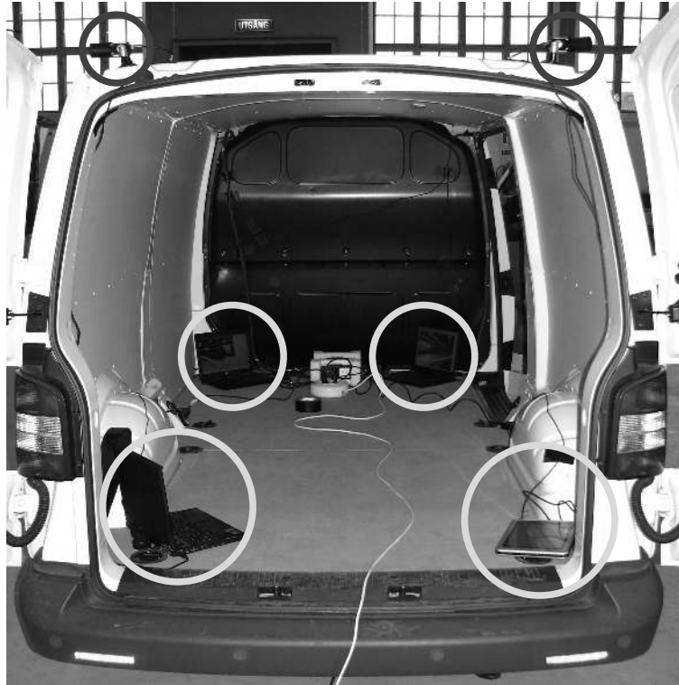
Figure 3: Test setup for the field trials. Within the dark circles are two of the four cameras mounted on the roof of the van. Each camera were connected to a laptop computers which were placed in the cargo compartment (grey circles)
