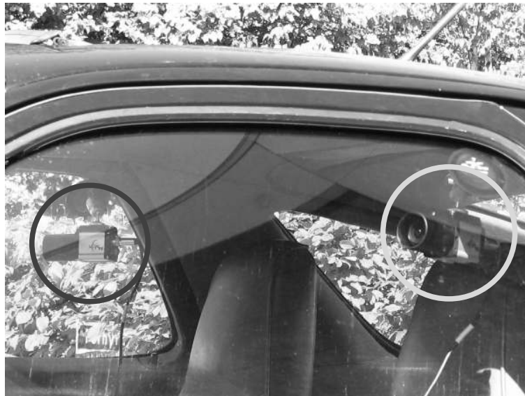
Figure 4: uEye cameras mounted on each side window of test vehicle during initial field trials.
