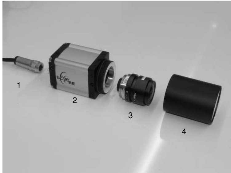
Figure 2: Exploded view of uEye camera; USB cable and connector (1), camera housing (2), lens (3), and lens cover (4)
