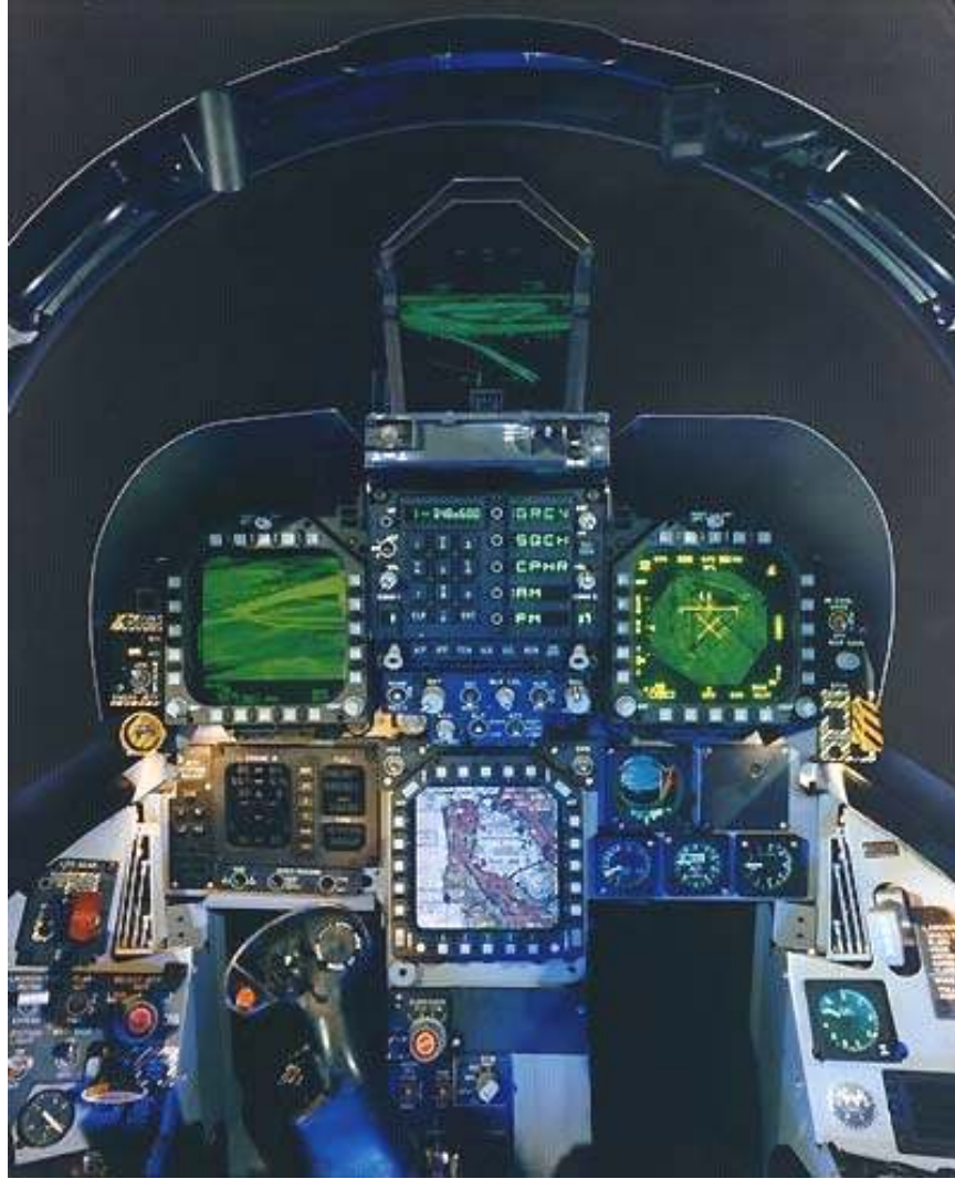
Figure 4: F18 C/D cockpit showing the complex array of visual instruments.
