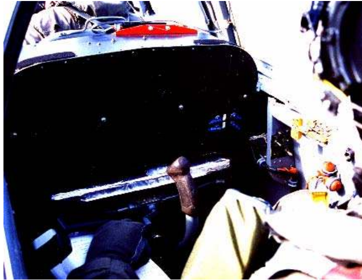
Figure 17: NT-34C, “266” rear cockpit showing absence of visual instruments.
