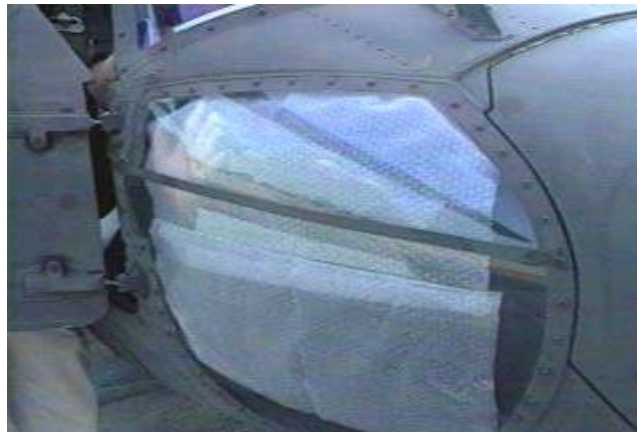
Figure 37: UH-60 chin bubble with opaque plastic lining.
