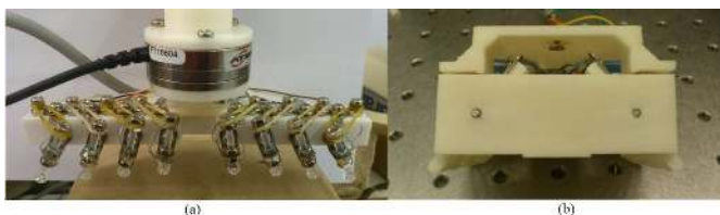
Fig. 16. Photos of (a) “spider” and (b) “spider2” sensors. Senses friction ranges by detecting which legs (arranged at different angles) slip when pressed against a planar object. Reproduced from [104] with permission from Springer, Copyright 2016.
