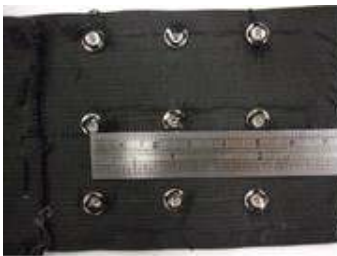
Fig. 1. The 3x3 tactor array with an inter-element spacing of 25mm
