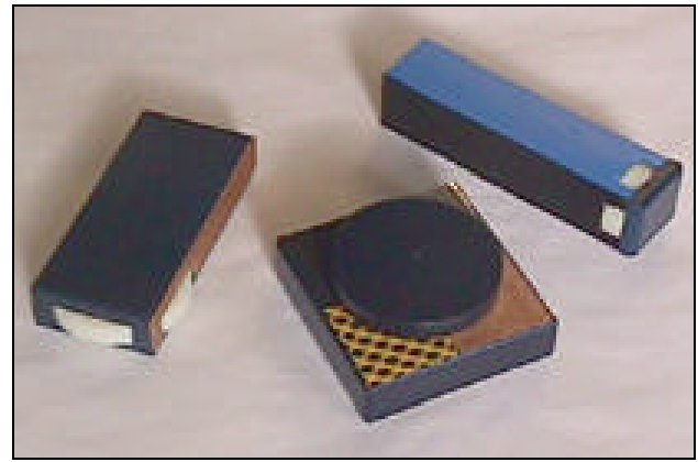
Figure 10: Conceptual side-selection prototypes. The force-feedback wheel’s mode is chosen by pressing the wheel at a specific position (left and right prototypes) or a position on the wheel’s base (center). Since activation location is grounded relative to hand position, the selector is easy to find.
