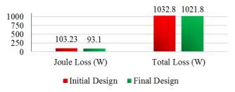
Figure 8. Comparison between Joule loss and total loss in the initial and the final design of HS-PMSG.
