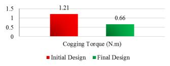
*Figure 9.* Comparison between cogging torque in the initial and the final design of HS-PMSG.
