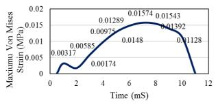
Figure 11. Maximum Von Mises strain in the rotor.
