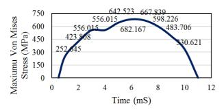
Figure 10. Maximum Von Mises stress in the rotor.
