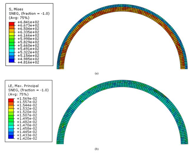
Figure 4. FEM analysis of the final design of HS-PMSG, Von Mises stress (MPa) (a) and Von Mises strain (MPa) in the PM and the retention sleeve (b).
