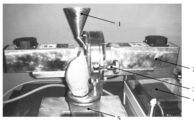
Figure 1. Laboratory device for mechanical activation of geomaterials: 1—hopper for the initial material; 2—disintegrator section with the electric motor; 3—clamping device; 4—control block; 5—storage capacity.
