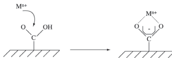
Scheme 1. Cation exchange mechanism with the carbon surface carboxylic groups.
