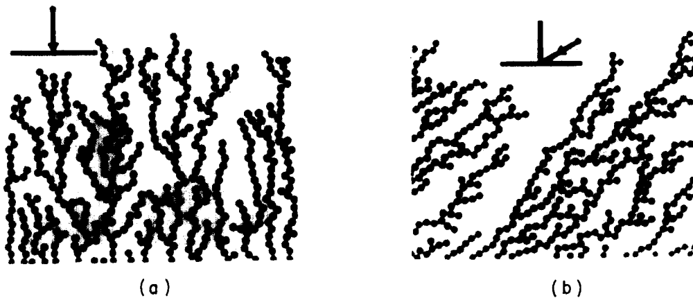
Fig. 13. 2-D simulation of growth under (a) normal and (b) oblique incidence angles. No relaxation was allowed. In (a) the chain-like structure is nominally perpendicular to the substrate, whereas in (b) it is inclined at an angle between the film normal and the incidence angle [37].
