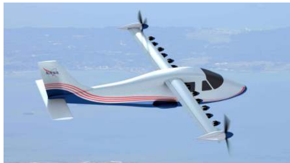
Fig. 1 NASA X-57 thin-haul concept aircraft illustration* showing the mid span DEP propellers in the folded cruise position.
