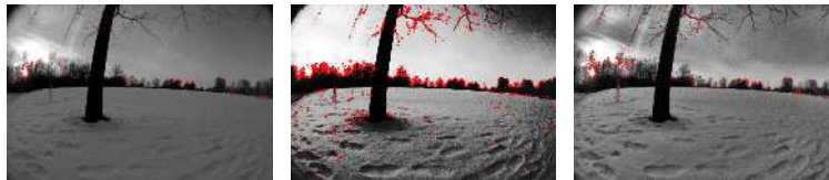
Fig. 2 Comparison of FAST features detection on (a) a normal image, (b) image enhanced by global histogram equalization, (c) image enhanced by CLAHE.
