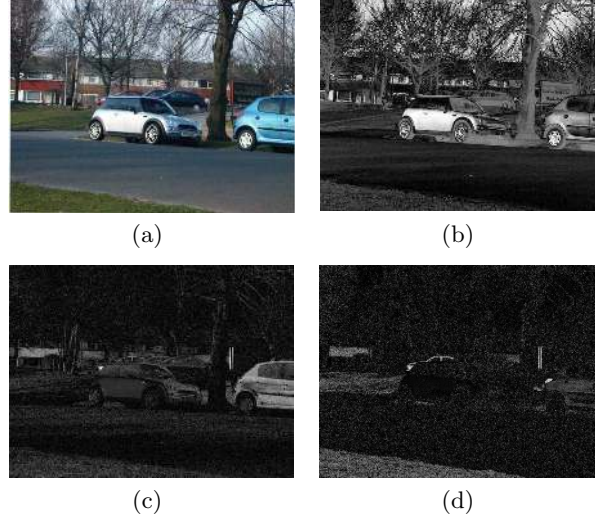
Fig. 6. PCA of an uncompressed image. (a)an uncompressed color image. (b) first PCA component of (a). (c) second PCA component of (a). (d) third PCA component of (a).
