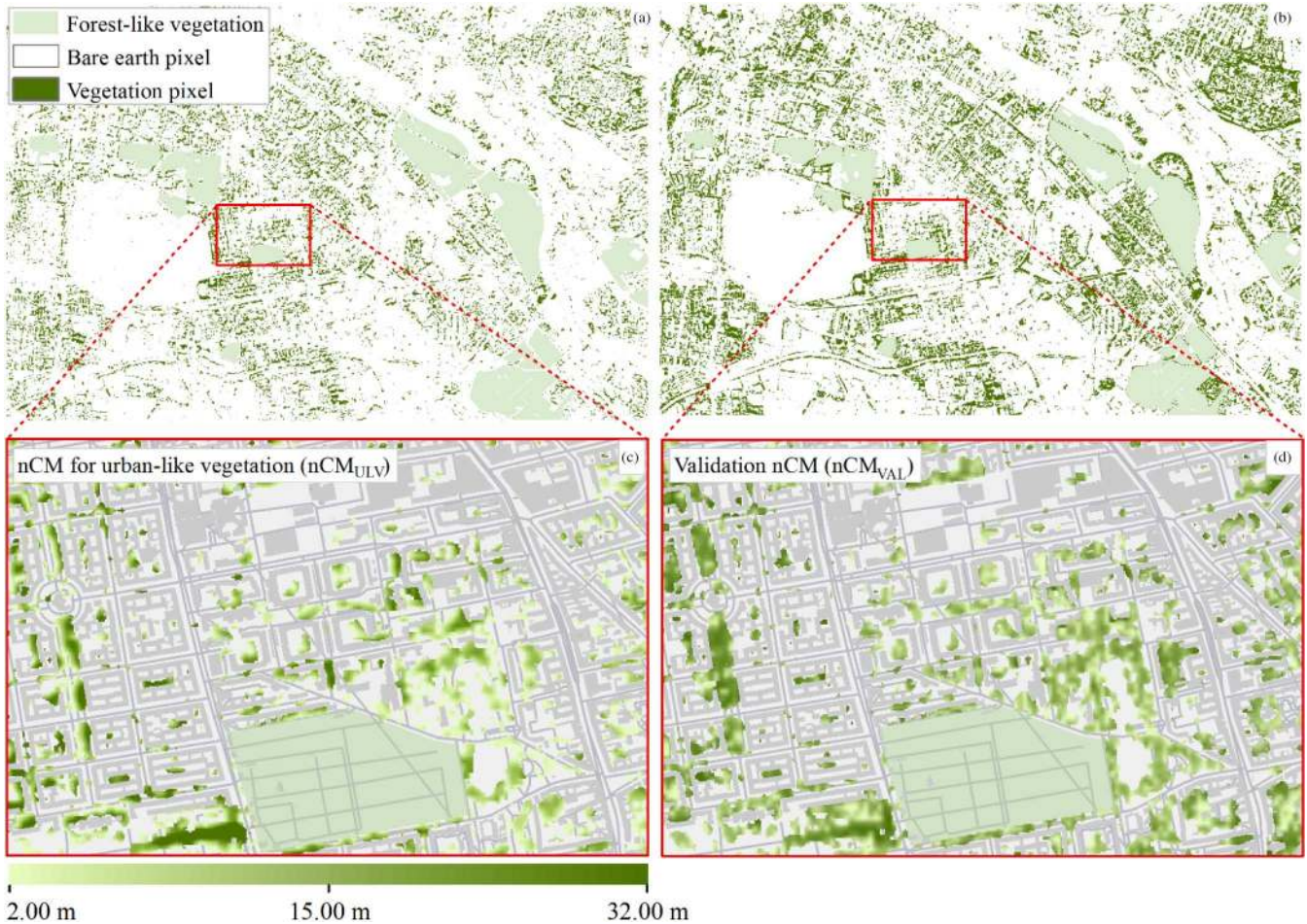
Fig. 5. Results of (a) DPMF-filtering in comparison to (b) UltraCam vegetation layer; and (c) nCM for urban-like vegetation in comparison to (d) validation nCM.
