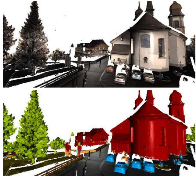
Figure 1. Convolutional networks based on tangent convolutions can be applied to semantic analysis of large-scale scenes, such as urban environments. Top: point cloud from the Semantic3D dataset. Bottom: semantic segmentation produced by the presented approach.
