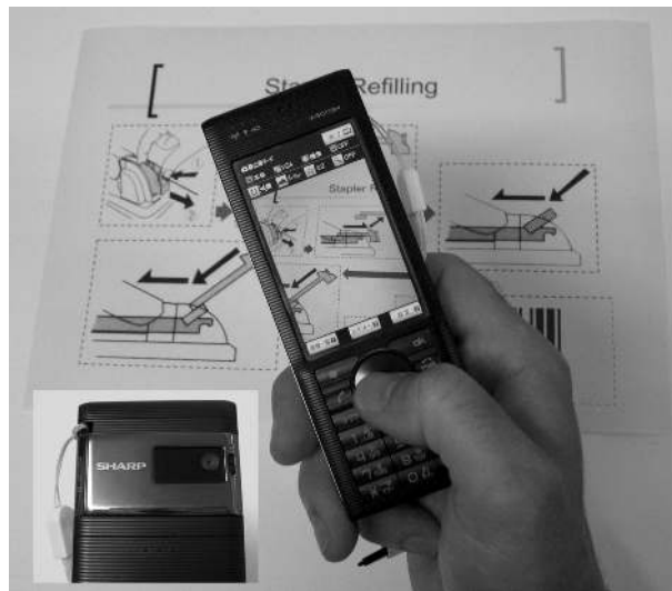
Fig. 7. An integrated Windows Mobile based communication device with an embedded camera.
