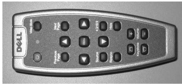
Fig. 1. Projector remote control unit with presentation control buttons.
