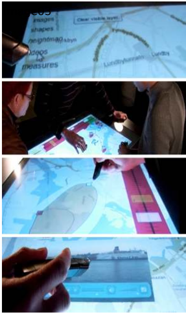
Figure 3 (top to bottom): The system offers interaction with five global layers (images, shapes, height map, videos, and measures); a specific layer is selected using the pen. Standard operations like placement of operational ERM units, such as a police car, a fire fighter, or a photographer, is activated using the “images” layer. The shape layer allows users to draw and modify time-dependent freeform areas. The video layer offers live streaming of video from an incident location.
