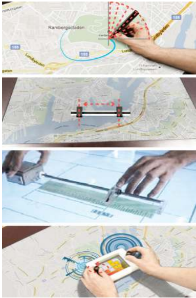
Figure 5 (top to bottom): We envision three new tool concepts where more precise device tracking and devices with a higher degree of specialization could benefit input. For the pen, streaming of its tilt-data and tip pressure value could provide new input modes. For the timeline function, a new handheld tool with two connected handles could support intuitive control of upper and lower values interval (concept and earlier example [4]). In an extended version of the frame, two adjustable knobs could enable bi-factorial browsing of map-based data.
